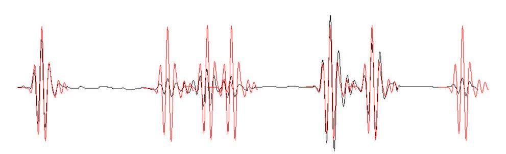
Templates shifted to best match the pulses using correlation of the template with the pulse.
