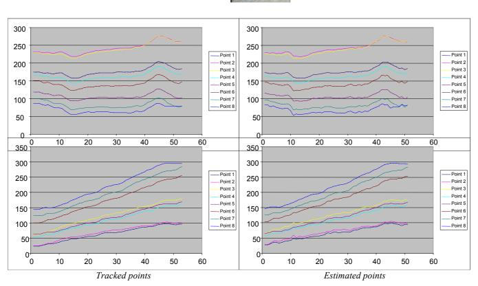
Estimation of 2D points positions from the estimated 3D transformation on the *Aerosonde sequence* (8 tracked points).
