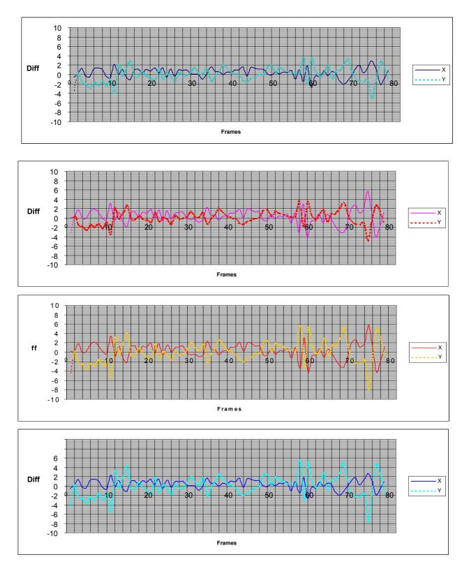
*Errors between the tracked points and the estimated points The increase in discrepancy towards the end of the sequence appears to be due to tracking error : it is something that needs investigating further*
