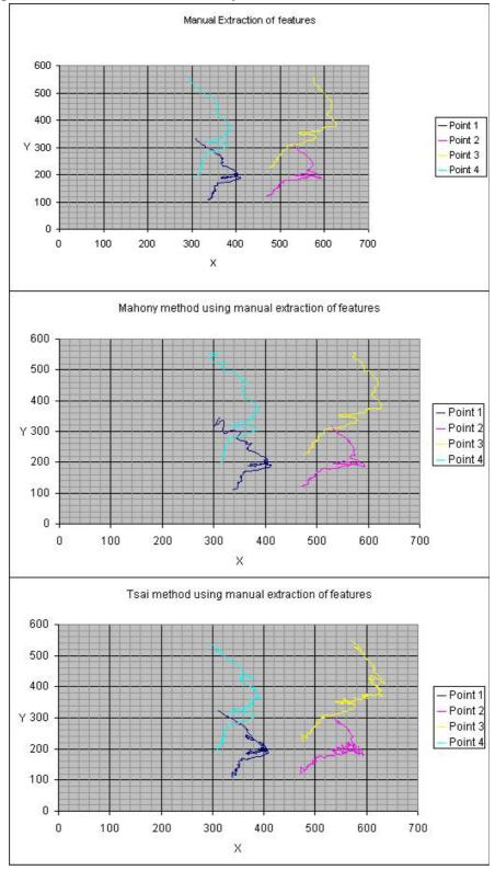
Estimated 2D point positions from the 3D transformation on the Aerosonde sequence
