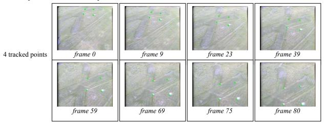
Successful corner tracking over the Aerosonde sequence (with a manual selection of features)
