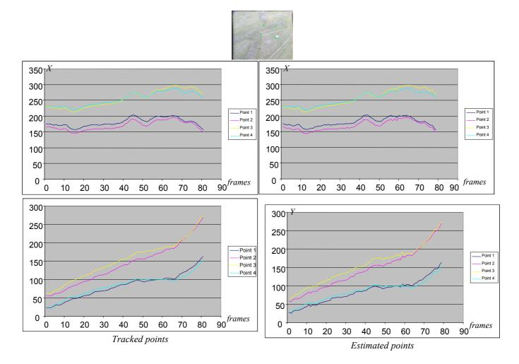
Estimation of 2D points positions from the estimated 3D transformation on the *Aerosonde sequence* (4 tracked points). This is one simple "sanity check" is to re-project and compare with the original tracked points.
