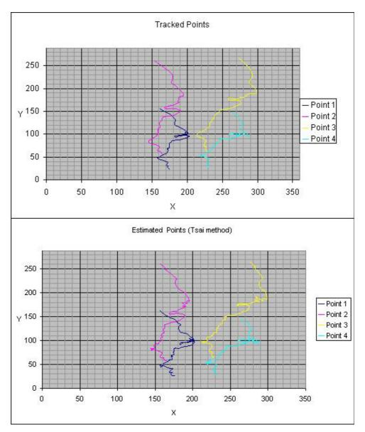
Estimation of 2D points positions from the 3D transformation on the Aerosonde sequence with Tsai method
