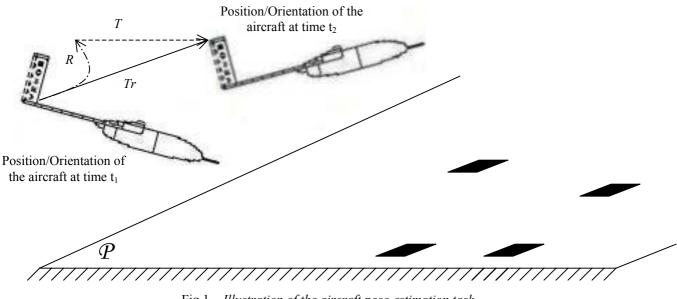
$Fig. 1-Illustration\ of\ the\ aircraft\ pose-estimation\ task$
