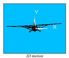
This last OpenGL representation shows the estimated pose of the aircraft over the sequence.
