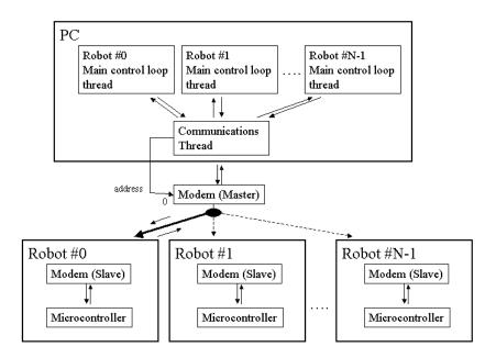
Fig. 3. Core components in the complete system design. Here, N is the number of robots.
