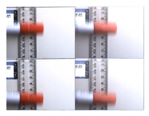
Figure 6.2: Consecutive frames of a pen being waved in front of two cameras located on the same FireWire bus.
