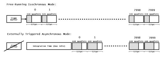
Figure 5.5: Difference in timing and bandwidth usage for normal 'free-running' isochronous and externally triggered asynchronous capture modes.
