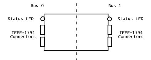
Figure 7.2: The Sync Unit bridges timing information across 2 buses.
