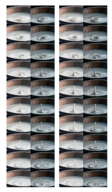
Figure 7.9: Milk drop tests 1 and 2. Left and Right: (Top to bottom) 10 consecutive frames of the result of a milk drop hitting a bowl of milk as captured by two colour cameras located on different host PCs and being triggered to capture isochronously over Ethernet.
