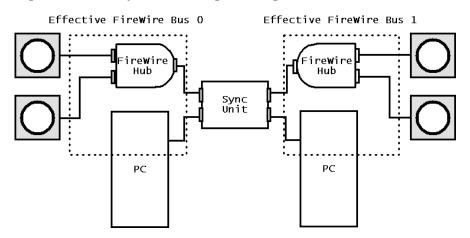
Figure 7.3: Synchronising 4 cameras across 2 buses using the Sync Unit.
