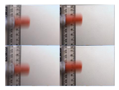
Figure 7.6: Consecutive frames of a pen being waved in front of two cameras attached to different host PCs and being triggered to capture isochronously over Ethernet.
