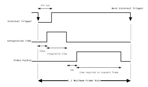
Figure 5.4: Timing of image acquisition when using an asynchronous external trigger. *Source:* [6], p. 24 (adapted)
