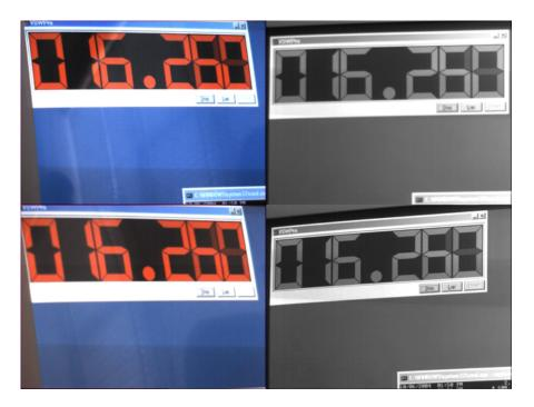
Figure 7.7: Stopwatch images from all 4 cameras for a frame near the start of capture. The top-left and bottom-left colour cameras are both located on the same FireWire bus on one host PC. The top-right and bottom-right mono cameras are both located on the same FireWire bus on a different host PC.
