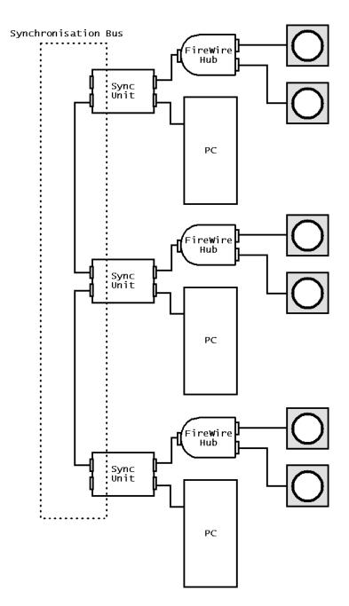
Figure 7.4: Synchronising 6 cameras across 3 buses by daisy-chaining 3 Sync Units.
