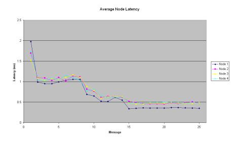
Figure 7.5: Average one-way latency times observed for UDP messages between server and client.
