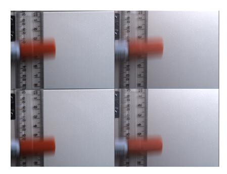
Figure 5.2: Consecutive frames of a pen being waved in front of two cameras being triggered externally.
