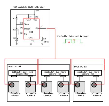
Figure 5.1: Externally triggering 6 cameras located on 3 FireWire buses across 2 PCs.
