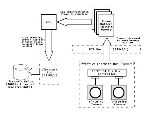
Figure 4.1: Flow of video data from camera to disk.
