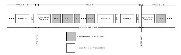
Figure 2.1: Timing of multiple isochronous and asynchronous data transfers. *Source:* [1], p. 155 (adapted)
