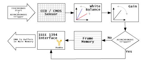
Figure 5.6: Flow diagram for normal isochronous and externally triggered asynchronous modes.
