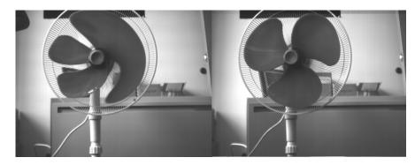
Figure 3.2: Left: Motion blur exhibited by CMOS rolling shutter. Right: Same scene imaged by CCD global shutter. *Source:* Point Grey Knowledge Base Article 115.
