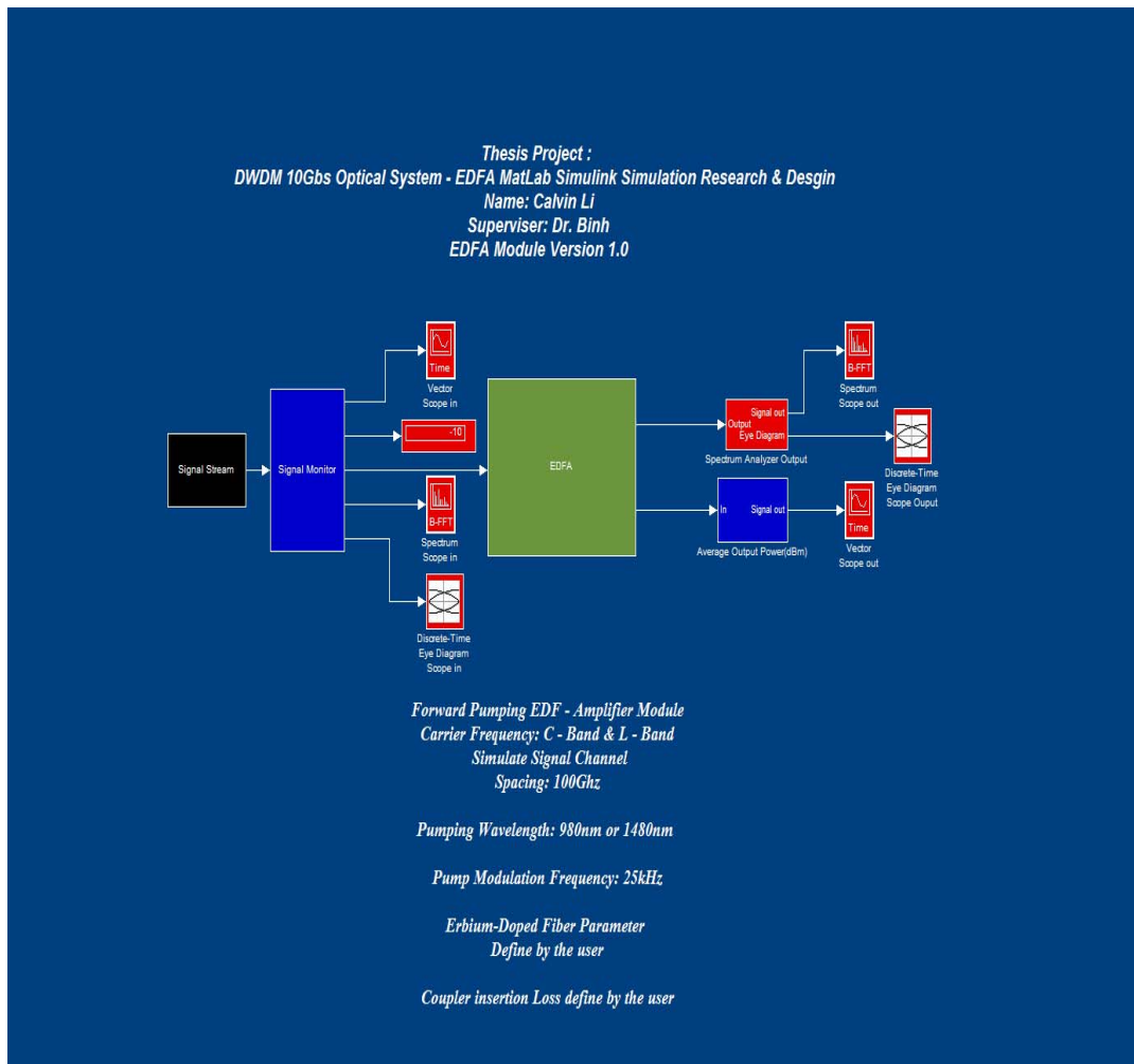
Figure 14 EDFA Module amplifier and monitoring systems.
