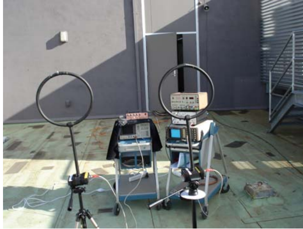
Figure 5. Calibrating the loop antennas.
